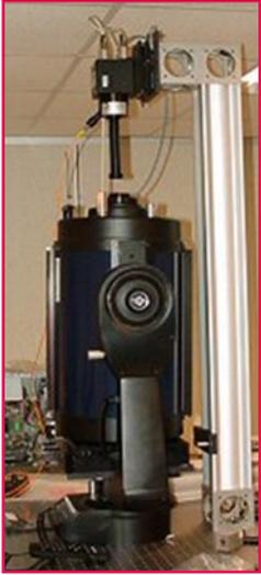
The diagram below shows an easy to configure method for measuring the wavefront error (WFE) of a Schmidt-Cassegrain telescope using an Imagine Optic HASO R-Flex 32 on a standard optical workbench. In this example, the source was adapted to the numerical aperture of the telescope by using a standard  $f/10$  objective.
